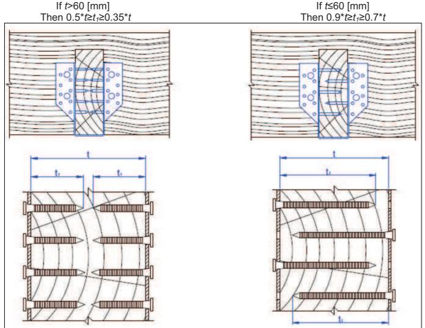
Figure 37 Rule for placement nails
